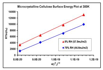
Figure 5. Dispersive surface energy plots for MCC at 0 and 70% RH.
