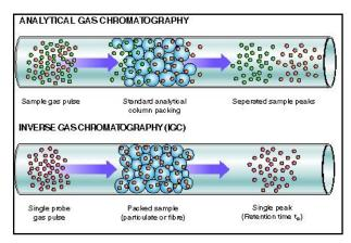
Figure 2. Schematic of IGC principle.
