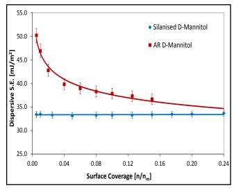
Figure 8. Dispersive surface energy profiles (as a function of surface coverage).
