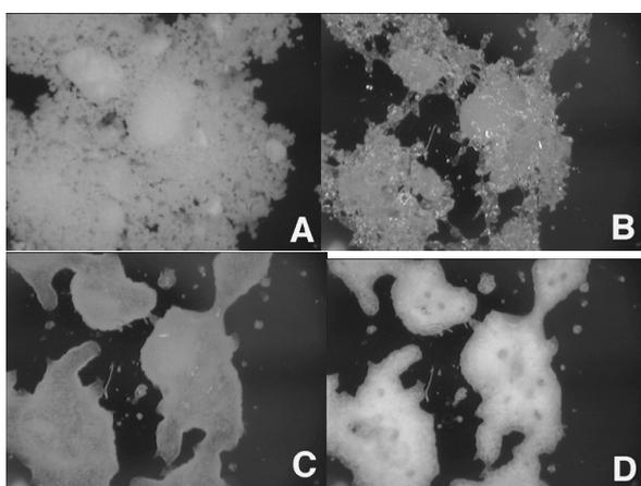
Figure 10. In-situ images collected on amorphous lactose at 0% (A), 50% (B), 60% (C), and 90% RH (D).
