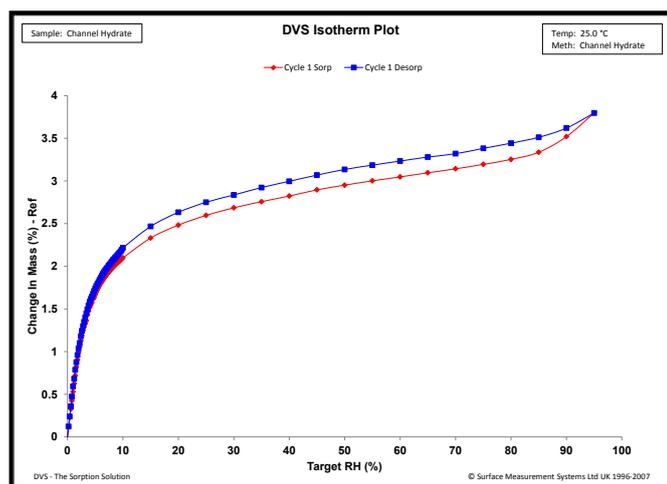
Figure 4. Water sorption kinetics Compound X at 25.0 °C.
