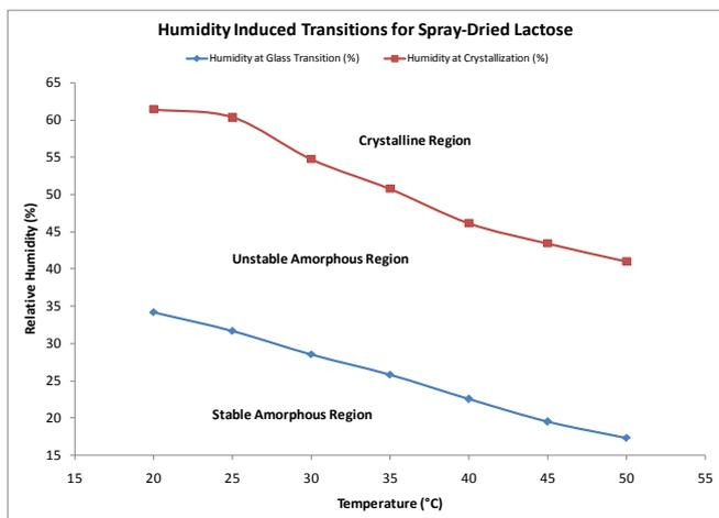
Figure 8. Humidity-induced phase transitions for spray-dried lactose measured via DVS.
