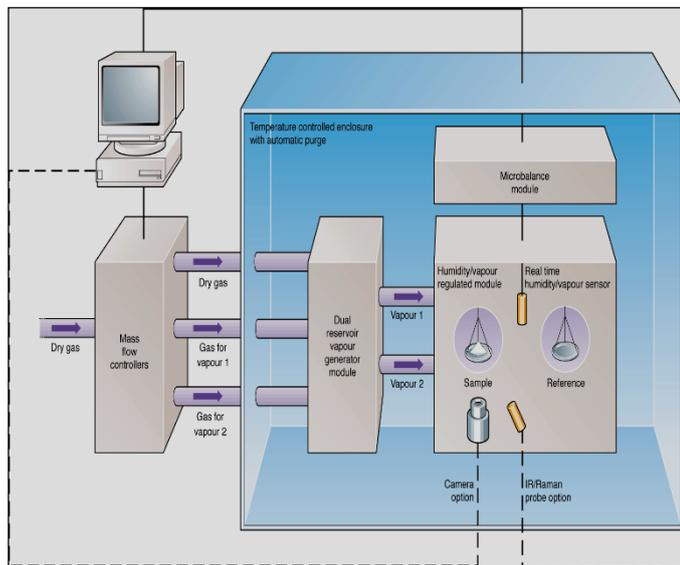
Figure 1. Schematic overview of the SMS DVS-Advantage instrument.
