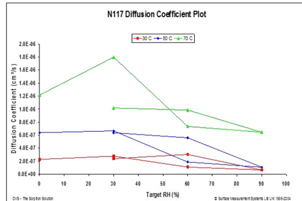
Figure 12. Diffusion coefficients at 30 °C (red), 50 °C (blue), and 70 °C (green) for a fluoropolymer-copolymer film (183 microns).
