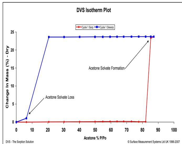
Figure 5. Acetone vapour sorption (red) and desorption (blue) isotherms for carbamazepine at 25 °C.
